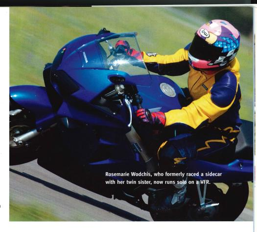
indication of the '94 model's considerably improved performance. A new exhaust system, intake porting and flat-slide carbs helped make 96 hp at the rear wheel, 8 hp up on the last model, and aided by a 10 kg (22 lb) weight reduction, the third-generation VFR wasn't far off the pace of the pure-sport 750s. A bigger 21 L tank also increased fuel range.
